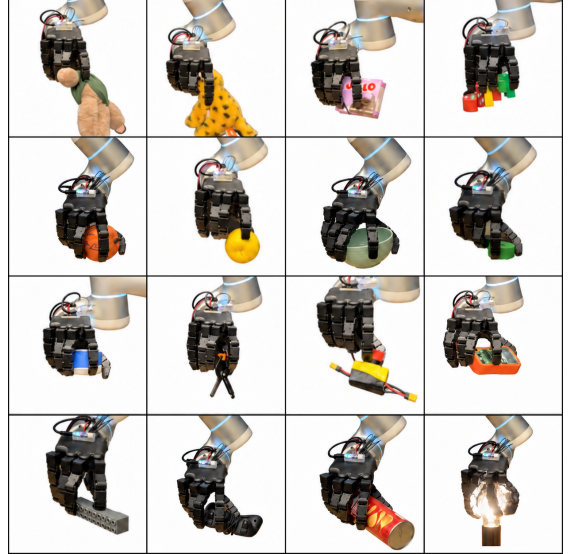
Fig. 1. The proposed method can grasp a diverse set of real world objects blindly without visual observations and priors.
